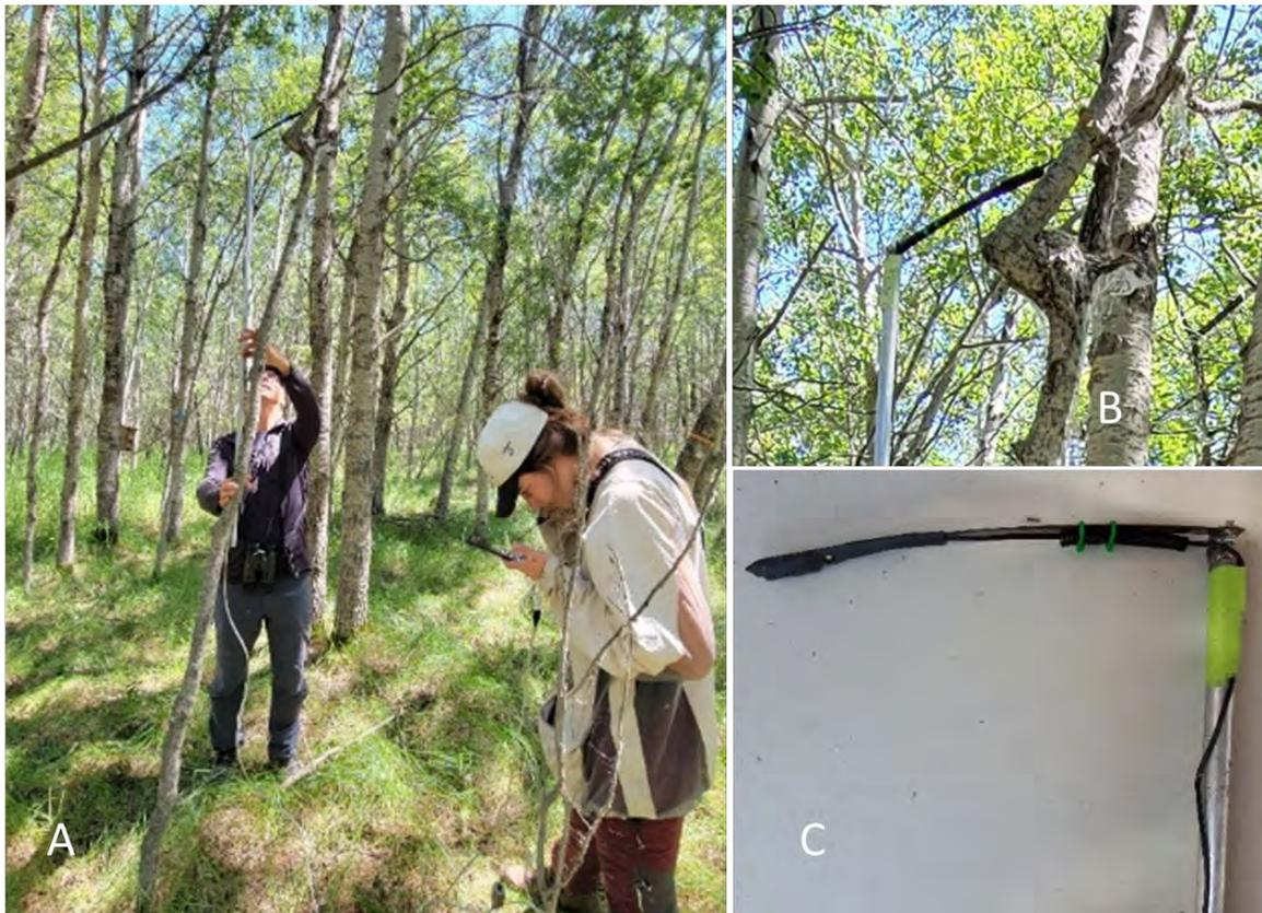
Figure 7: (A) Monitoring a nest with the pole camera connected to a smartphone. (B) Close-up of the pole camera above the nest. (C) Pole camera head.
