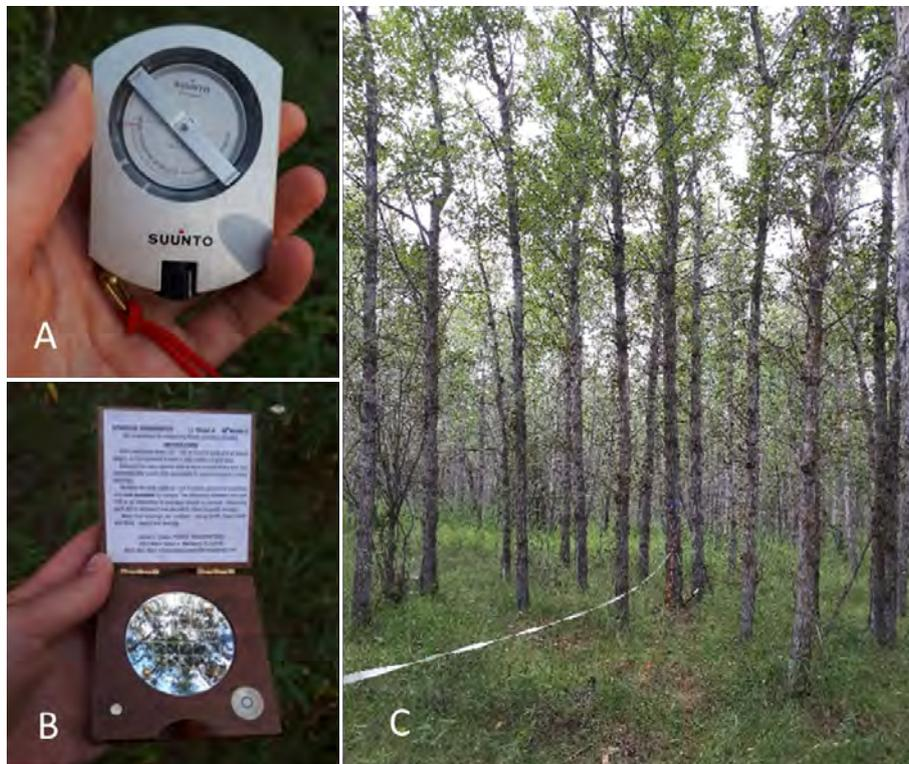
Figure 8: (A) Clinometer, (B) Densiometer and (C) plot of 5 m radius around nest tree with blue flagging.
